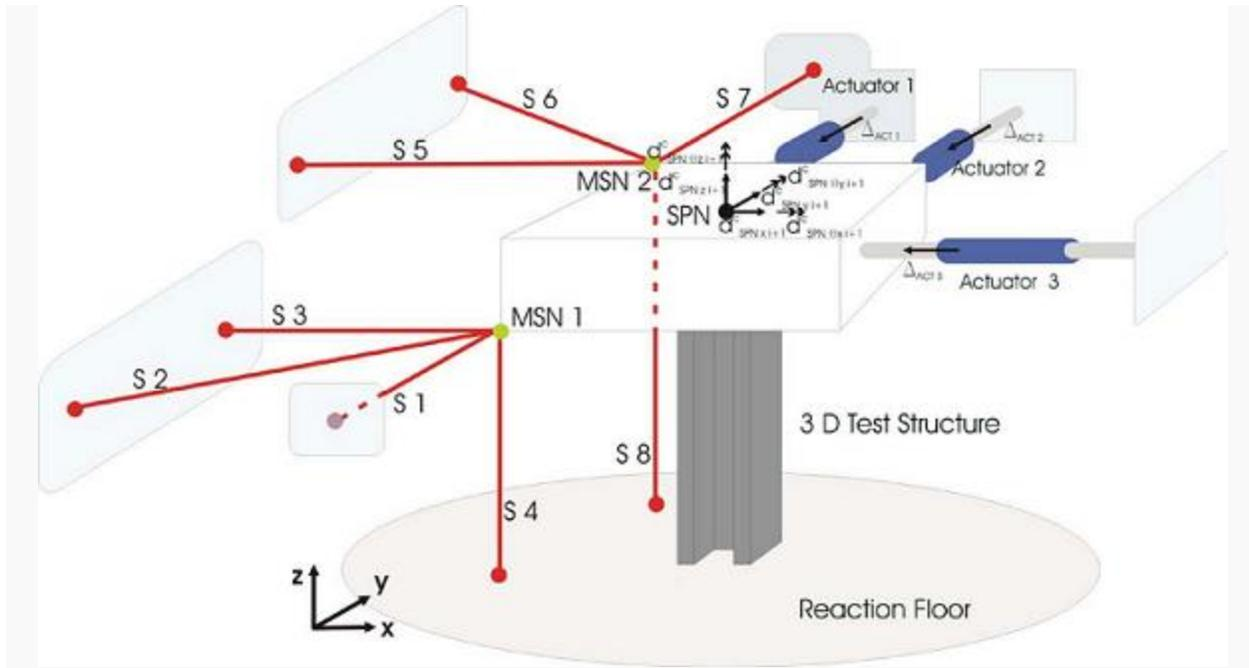
Figure 2-5 3-D test with displacement sensors arranged for tracking specimen position
