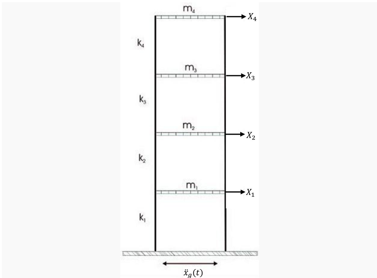
Figure 2-1 Shear building subjected to earthquake ground accelerations
