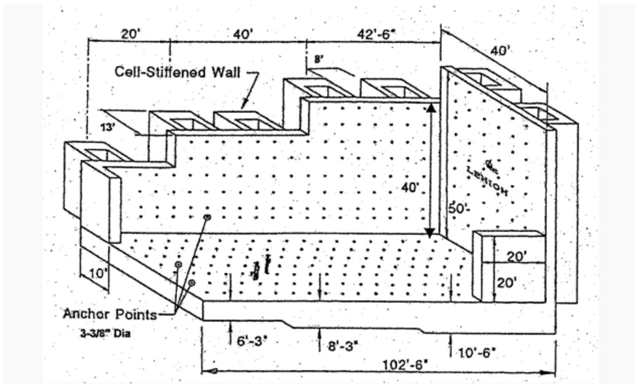
Figure 1-3 Multi-directional reaction wall and strong floor - isometric view
