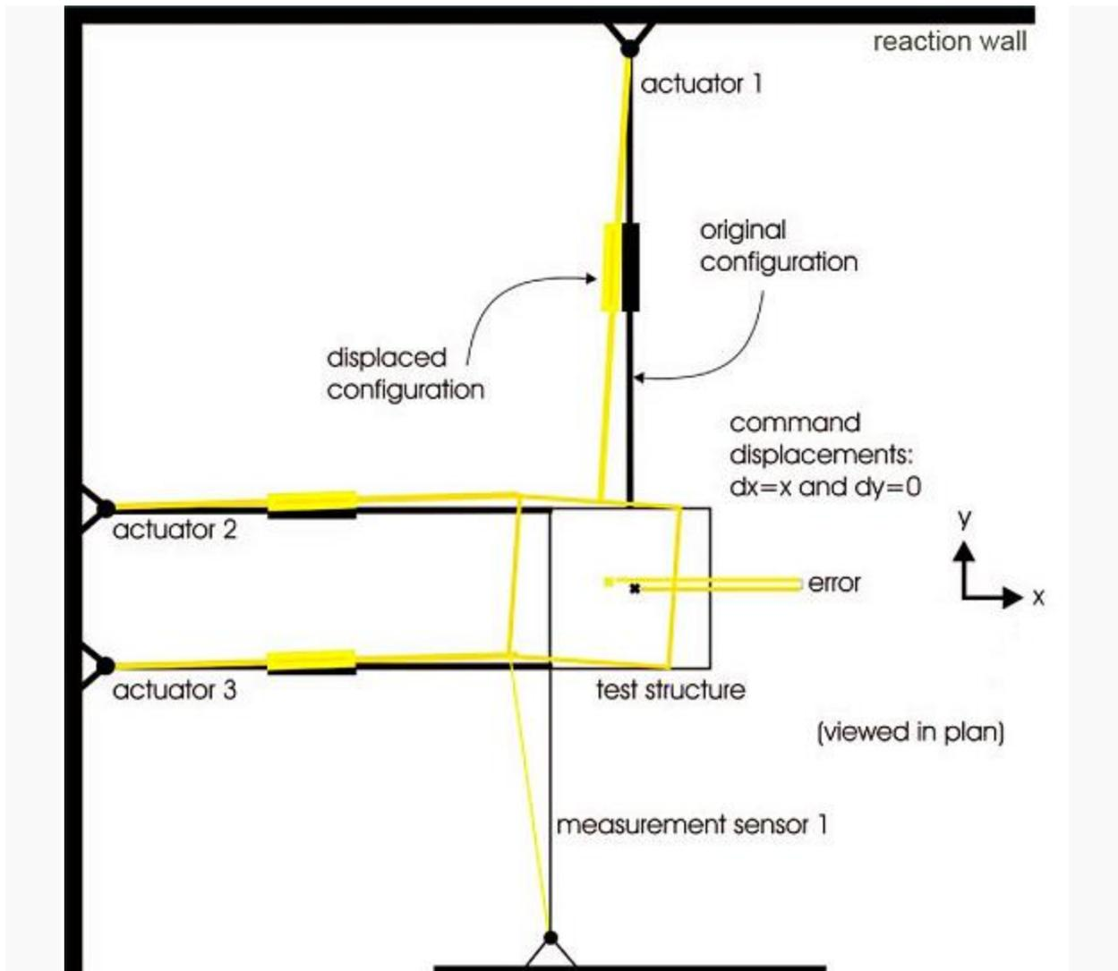
Figure 2-4 Geometrical inaccuracies due to test structure kinematics
