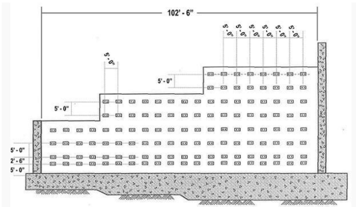
Figure 1-6 ATSS West Reaction Wall Elevation
