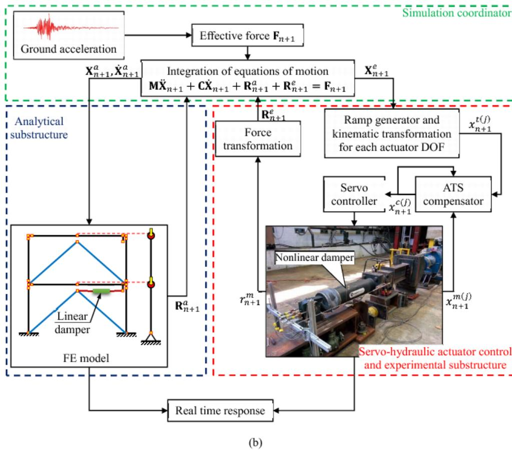
Figure 2-2 Real-time hybrid simulation: (a) example structural system subjected to seismic excitation, and (b) schematic representation of real-time hybrid simulation for the example structural system (Kolay, 2016).
