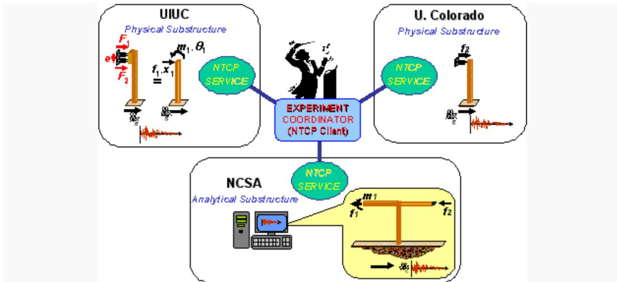
Figure 2-3 Distributed hybrid PSD testing: NEES MiniMOST experiment (Pearlman, et al. 2006)
