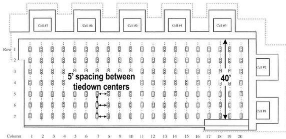
Figure 1-5 Floor Plan of Strong Floor
