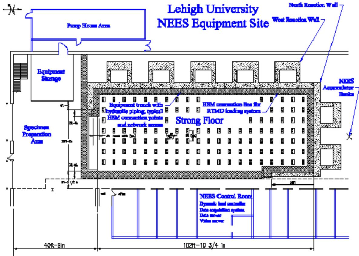
Figure 1-4 Floor Plan of RTMD Facility
