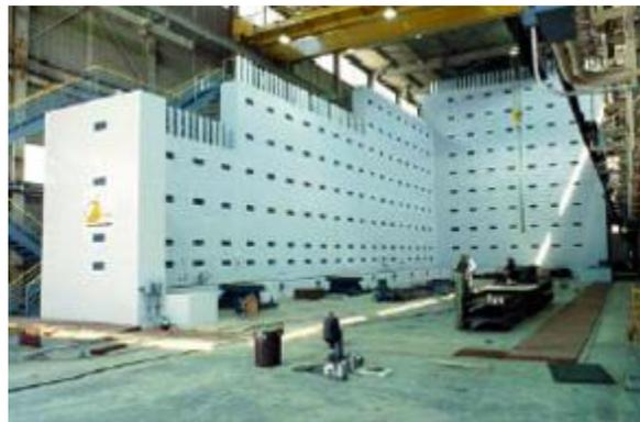
*Figure 1-1 ATLSS Multi-directional reaction wall*
