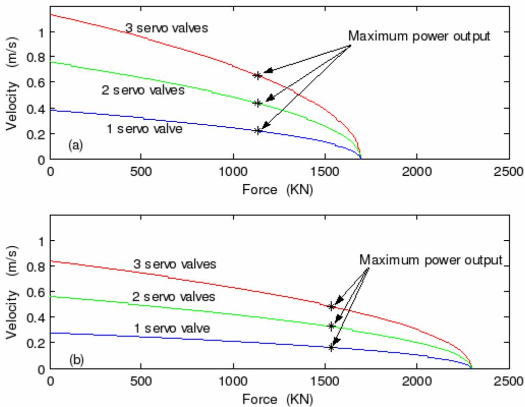
Figure 1-2 Hydraulic actuator power envelop for (a) 1700 kN actuators, and (b) 2300 kN actuators (20.7 MPa supply pressure)
