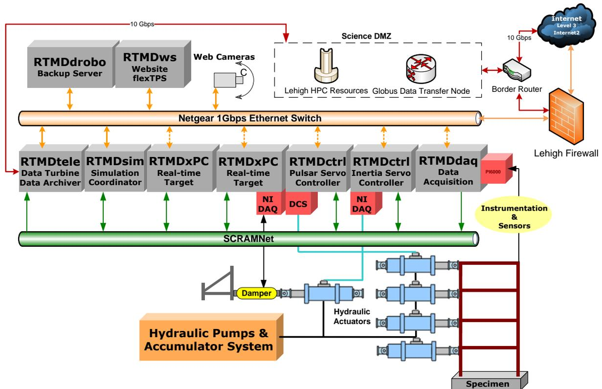
Figure 1-12 RTMD servo-hydraulic control and IT Infrastructure
