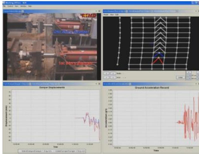
Figure 3-3 Screen capture of RDV showing live video, 3D model and plotting data
