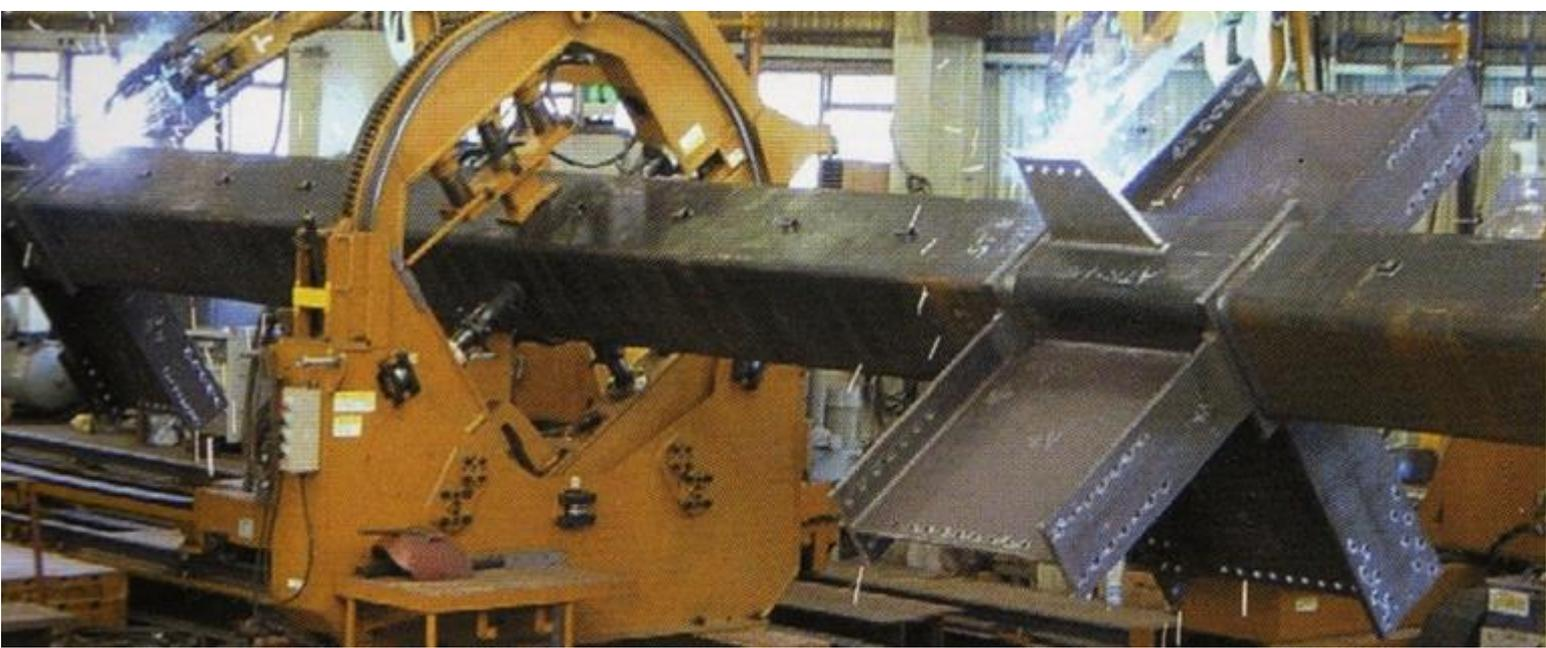
**Beam stubs that are welded to the column in the shop.**
