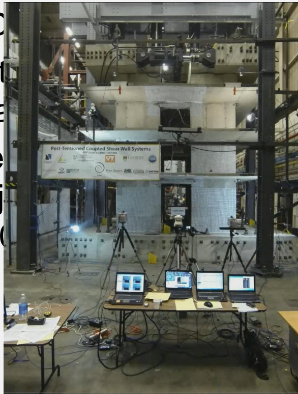
NEES@Lehigh Coupled Shear Wall Test Specimen with Multi-Directional Loading
