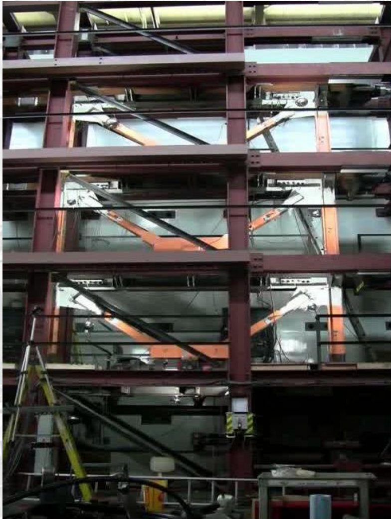
Experimental Substructure – CBF with MR Dampers
