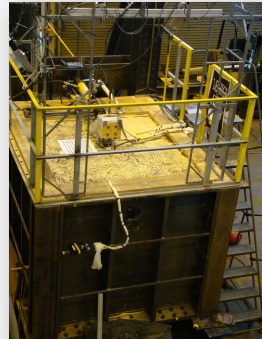
Pile Lateral Load Test
