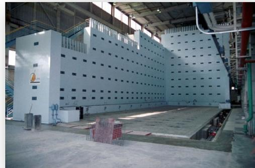
**Figure 3. ATLSS Center Multi-directional Reaction Wall and Strong Floor**
