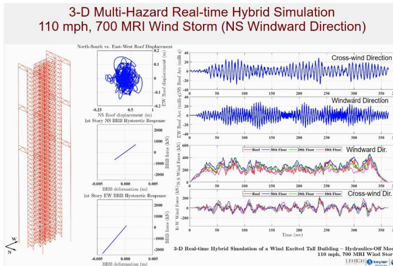
Figure 7. 3D Real-Time Hybrid Simulation of a 40-Story Building Subjected to Wind Hazards (Ricles & Cao, Lehigh University).
