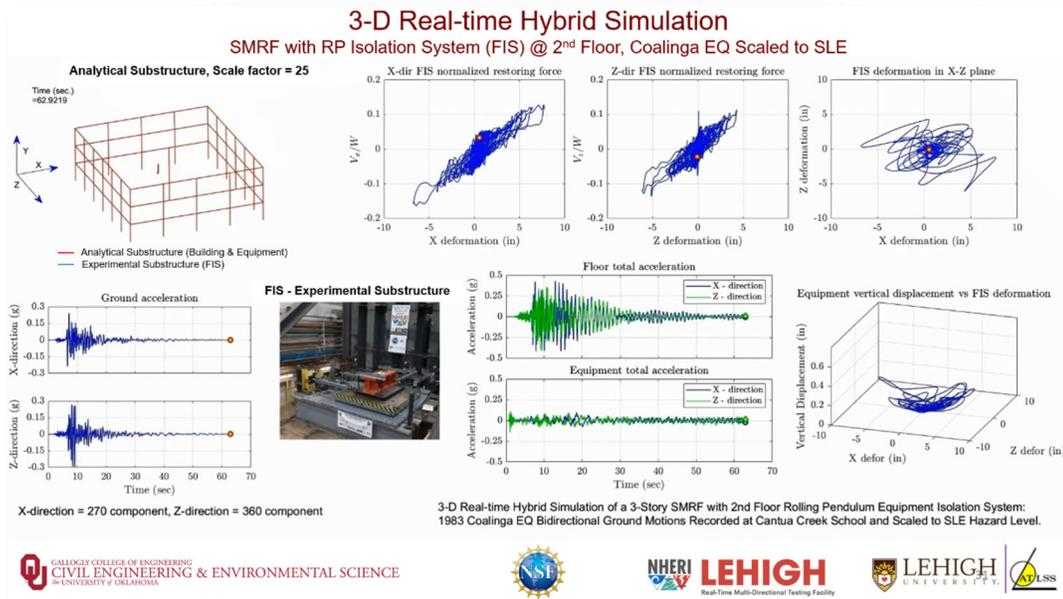
Figure 13. RTHS of FIS in moment resisting frames subject to multi-directional earthquake ground motions (Scott Harvey, University of Oklahoma).
