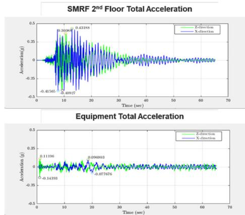
**Figure 14. RTHS Results: Illustration of the Reduction in Detrimental Equipment Accelerations By Using a FIS (Scott Harvey, University of Oklahoma).**
