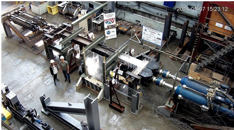
**Figure 11 Full-scale Investigation on the Performance of Seismic Collectors in Steel Building Structures: (a) Finite Element Modeling and Parametric Study; (b) 2-million Pound Test Setup for Full-scale Experiment Study (Robert B. Fleischman, University of Arizona).**
