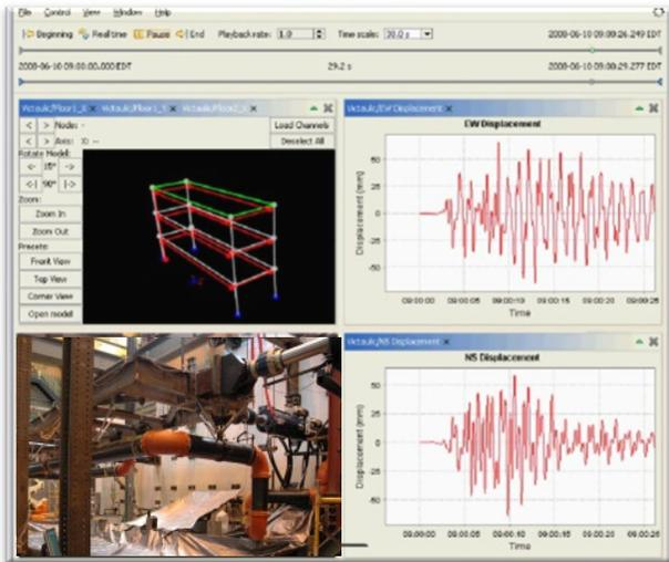
**Figure 8. 3D Large-scale RTHS of Building System Subject to Multi-directional EQ Ground Motions (Industry).**
