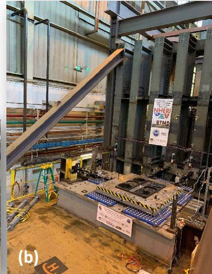
**Figure 2. Real-time Cyber-Physical Structural Systems Testing Laboratory: (a) Testbeds; and, (b) multi-directional shake table.**
