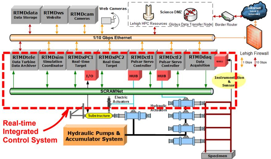
**Figure 5. Lehigh EF Real-time Integrated Control System**
