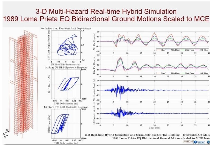
Figure 6. 3D Real-Time Hybrid Simulation of a 40-Story Building Subjected to Earthquake Hazards (Ricles & Cao, Lehigh University).
