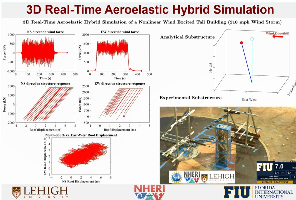
**Figure 15. 3D Nonlinear Real-Time Aeroelastic Hybrid Simulation of a Tall Building (Lehigh University and Florida International University).**
