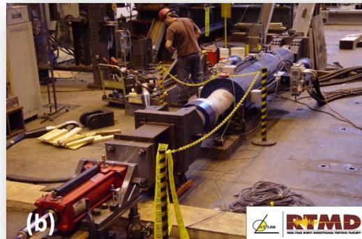
**Figure 10. Lehigh EF Large-scale (a) Self-Centering Lateral Force Resisting System (Richard Sause, Lehigh University), and (b) RTHS Semi-active Controlled Damper Testbed (Shirley Dyke, Purdue University).**
