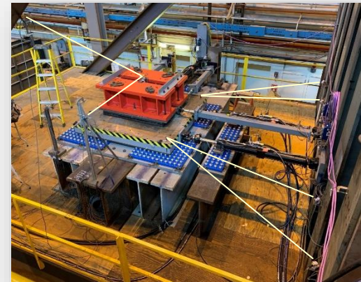
RTHS of Floor Isolation System using Multi-directional Shake Table
