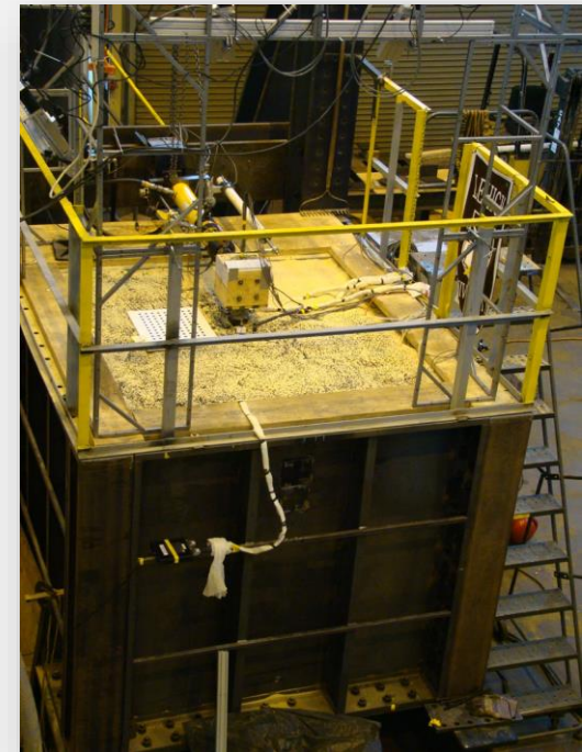
Pile Lateral Load Test
