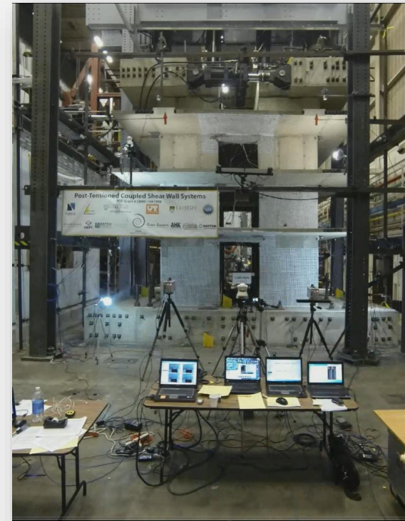
Characterization of Large-scale RC Coupled Shear Wall System Subject to Lateral and Gravity Loading
