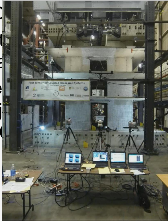
NEES@Lehigh Coupled Shear Wall Test Specimen with Multi-Directional Loading
