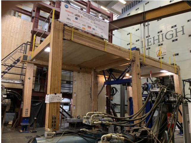
Large-Scale Multi-Directional Testing of a Cross-Laminated Self-Centering Shear Wall - Floor Diaphragm System under Simulated Earthquake Loading
