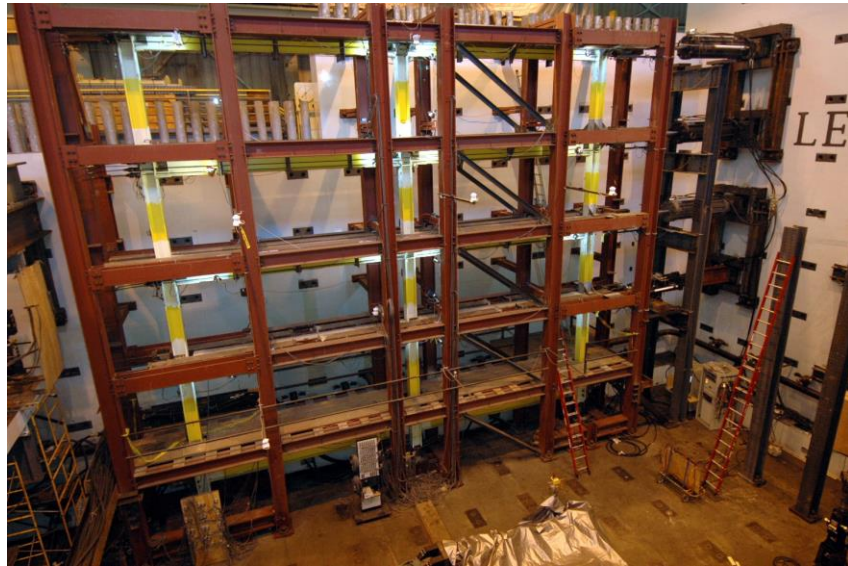
Large-Scale Hybrid Simulation of a Self-Centering Steel Moment Resisting Frame Building under Simulated Earthquake Loading
