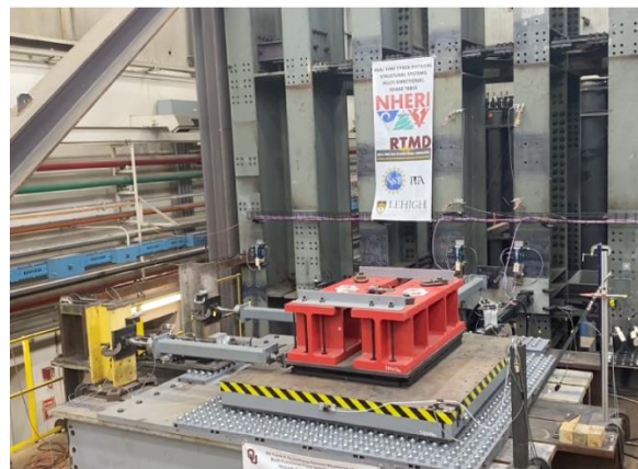
Test setup for multi-directional characterization tests and real-time hybrid simulations of floor isolation systems (R11 Track-4: Quantifying Seismic Resilience of Multi-Functional Floor Isolation Systems through Cyber-Physical Testing (OIA 1929151), PI - Scott Harvey, University of Oklahoma).
