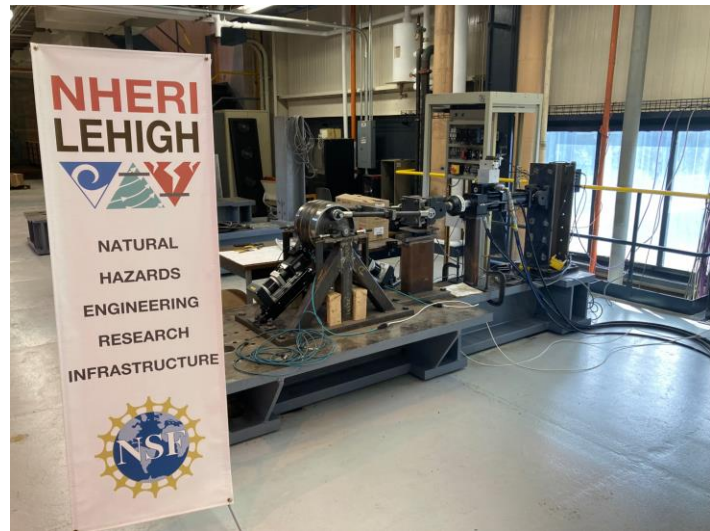
Cyber-Physical Structural Systems Testing Laboratory Testbed: characterization testing of a next-generation Banded Rotary Friction Damper for mitigating dynamic vibrations in structural systems.
