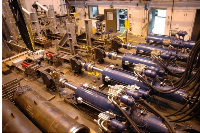
Large-Scale Damper Testbeds for Characterization and Real-time Hybrid Simulation of Structural Systems Subjected to Wind or Earthquake Loading
