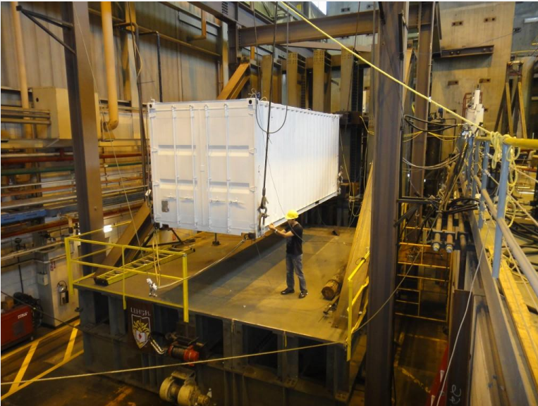
Test Setup with Cargo Shipping Container Debris
