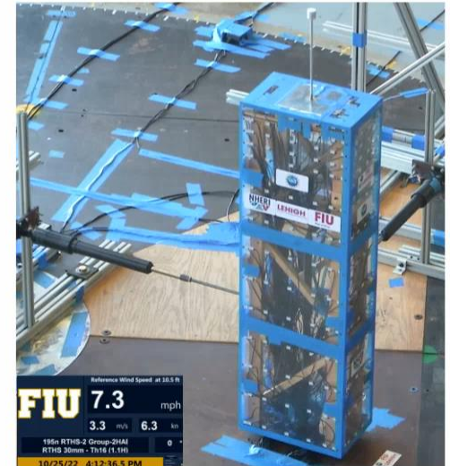
Experimental Substructure - RTAHS Building Model
