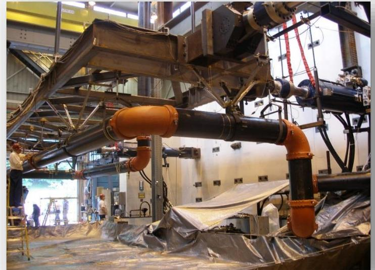
Multi-directional Dynamic Testing of Pipe Couplers
