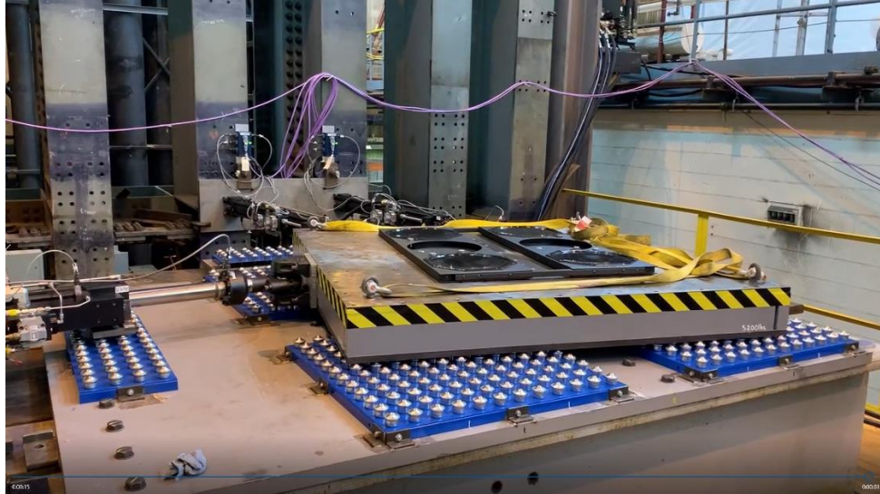
Figure 10. Photograph of completed multi-directional shake table with multi-directional translation and torsional in-plane motion applied.
