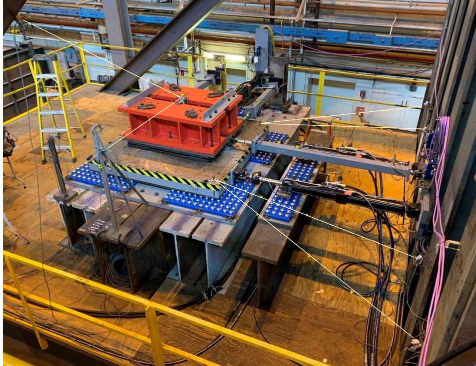
Figure 12. Real-time hybrid simulations of floor isolation systems (RII Track-4: Quantifying Seismic Resilience of Multi-Functional Floor Isolation Systems through Cyber-Physical Testing (OIA 1929151), PI - Scott Harvey, University of Oklahoma).
