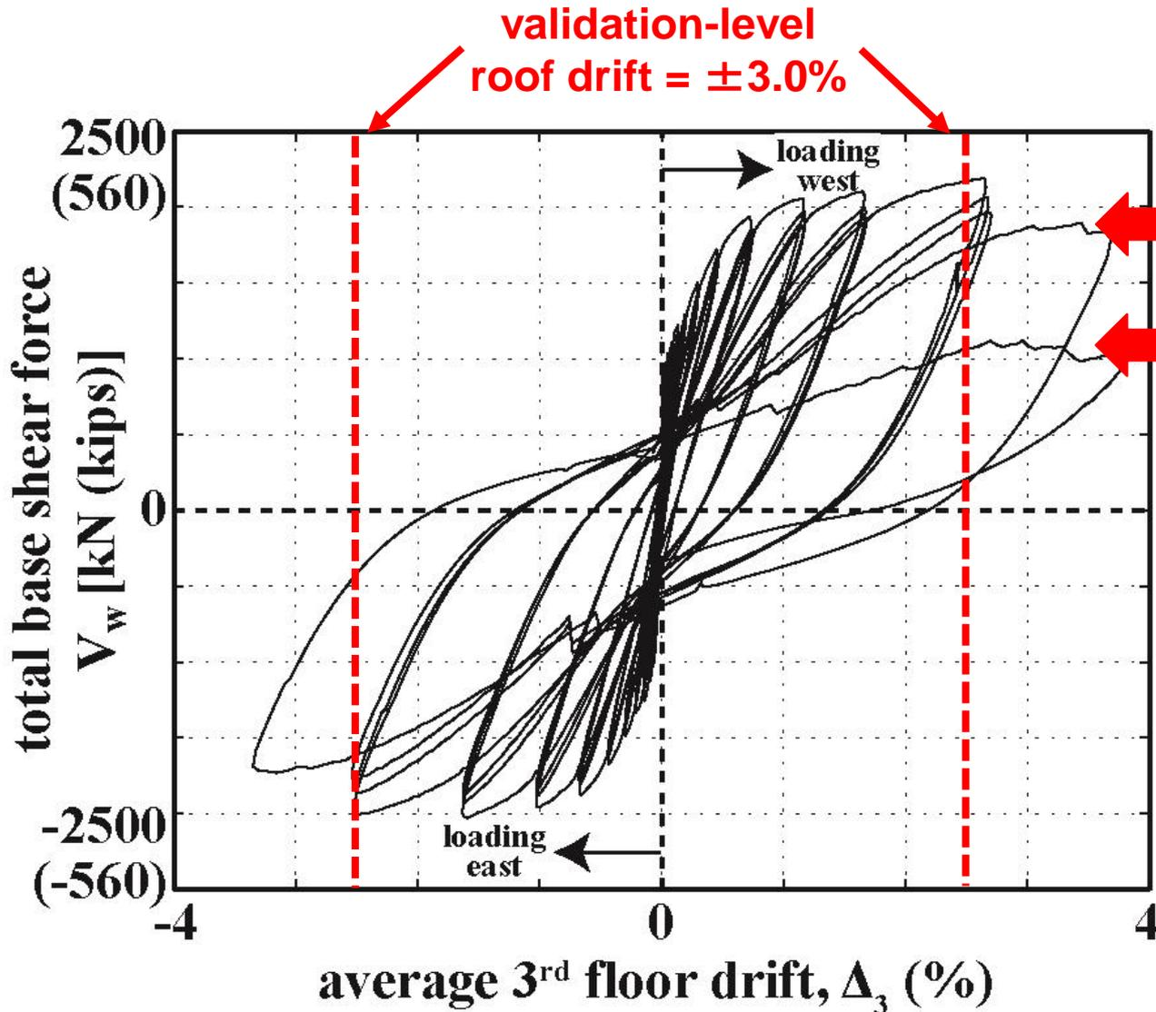
strength loss due to buckling+fracture of starter bars at flanges
