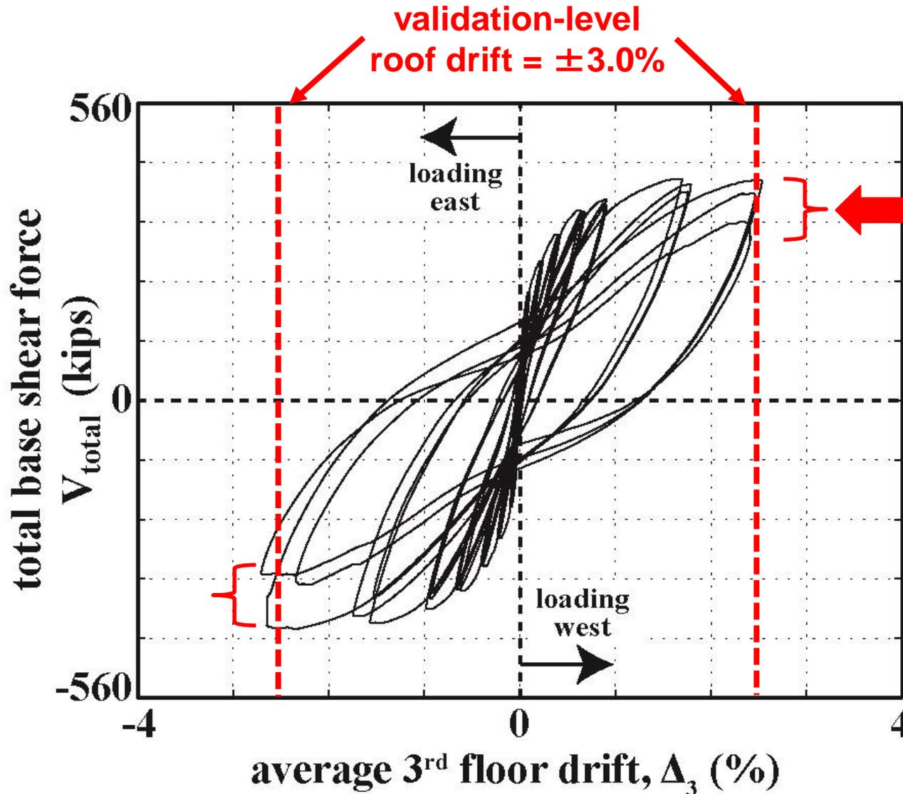
failure due to buckling+fracture of starter bars at toes
