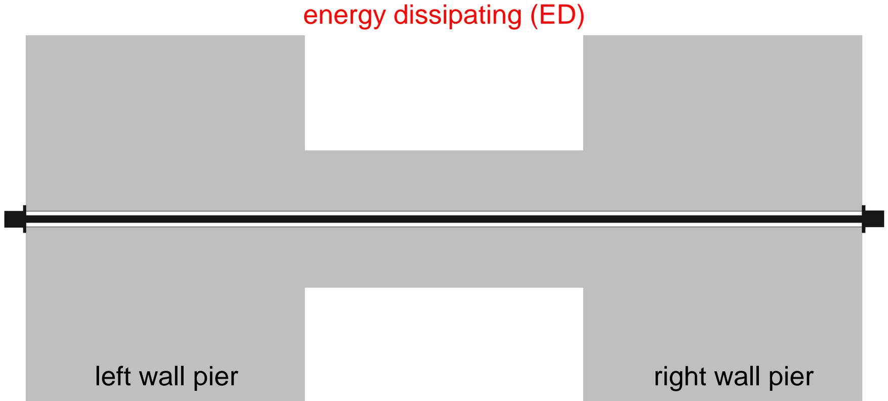
Partially Post-Tensioned RC Coupling Beam
