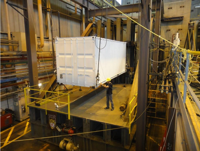
Test Setup with Cargo Shipping Container Debris
