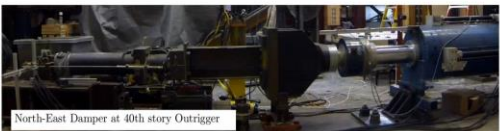
North-East Damper at 40th story Outrigger 3-D Real-time Hybrid Simulation of a Wind Excited Tall Building with NL Viscous Dampers Eastern 110mph, 700 MRI Wind Storm Experimental Substructure: Dampers
