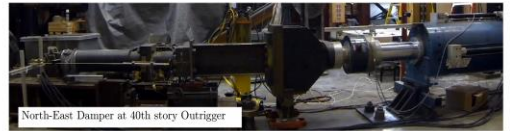
North-East Damper at 40th story Outrigger 3-D Real-time Hybrid Simulation of a Seismically Excited Tall Building with NL Viscous Dampers 1989 Loma Prieta EQ Bidirectional Ground Motions Scaled to MCE Level Experimental Substructure: Dampers
