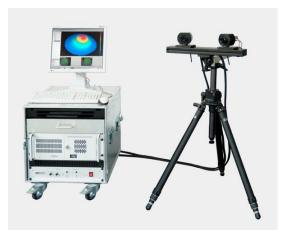
Figure 1-13 A complete Aramis system consists of an image processing computer and a pair of cameras
