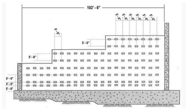
Figure 1-6 ATLSS West Reaction Wall Elevation
