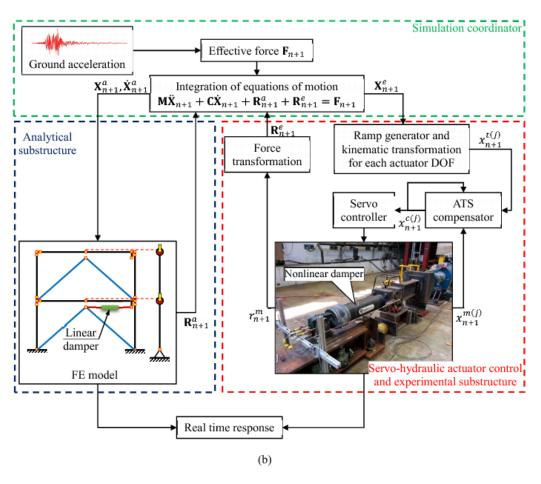
Figure 2-2 Real-time hybrid simulation: (a) example structural system subjected to seismic excitation, and (b) schematic representation of real-time hybrid simulation for the example structural system (Kolay, 2016).
