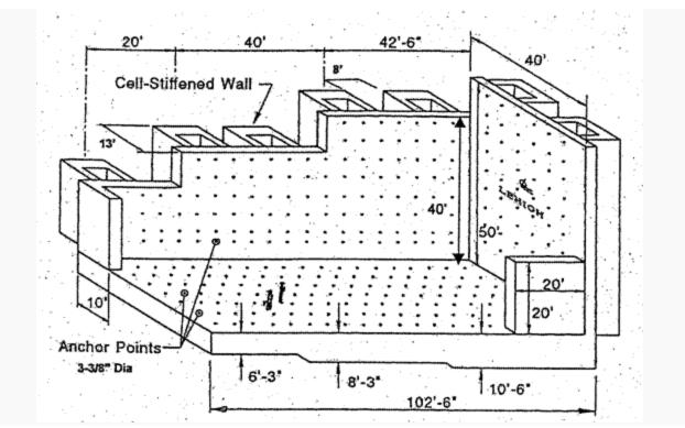
Figure 1-3 Multi-directional reaction wall and strong floor - isometric view
