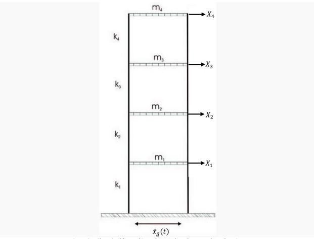
Figure 2-1 Shear building subjected to earthquake ground accelerations
