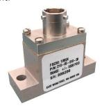
Figure 1-11 Differential Pressure Transducer
