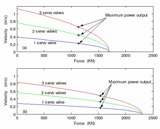
Figure 1-2 Hydraulic actuator power envelop for (a) 1700 kN actuators, and (b) 2300 kN actuators (20.7 MPa supply pressure)
