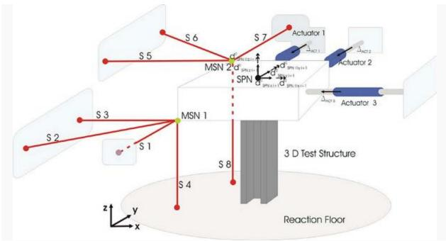
Figure 2-5 3-D test with displacement sensors arranged for tracking specimen position
