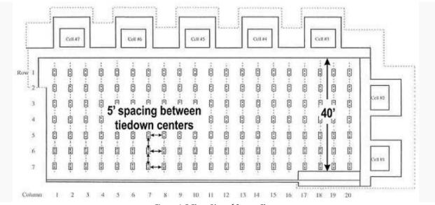
Figure 1-5 Floor Plan of Strong Floor
