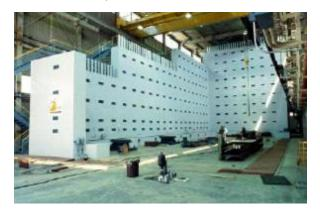
Figure 1-1 ATLSS Multi-directional reaction wall
