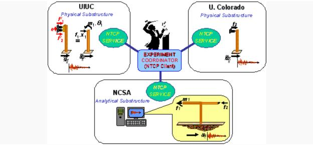
Figure 2-3 Distributed hybrid PSD testing: NEES MiniMOST experiment (Pearlman, et al. 2006)
