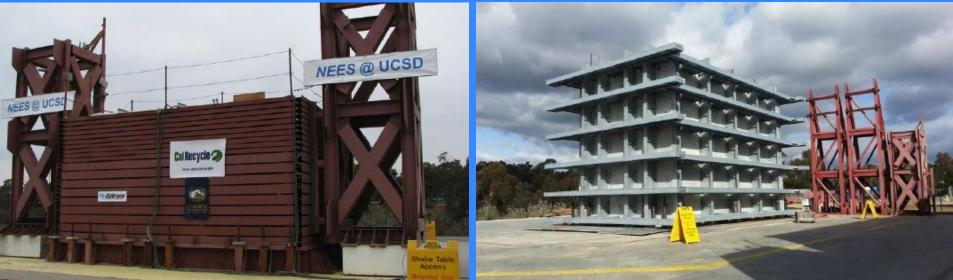
Laminar soil shear box:  $6.7m (L) \times 3.0m (W) \times 4.7m (H)$  Stiff soil confinement box: 10.0m (L)  $\times$  4.6 or 5.8m (W)  $\times$  7.6m (H)
