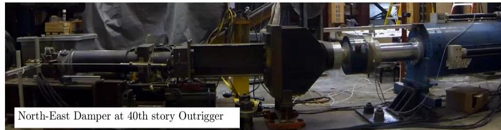
3-D Real-time Hybrid Simulation of a Wind Excited Tall Building with NL Viscous Dampers Eastern 110mph, 700 MRI Wind Storm
