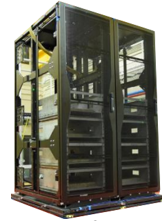
Server cabinet on top of RP isolation system
