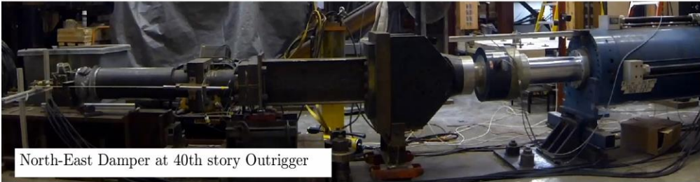
3-D Real-time Hybrid Simulation of a Seismically Excited Tall Building with NL Viscous Dampers 1989 Loma Prieta EQ Bidirectional Ground Motions Scaled to MCE Level
